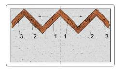
Start laying the first row of parquet from the center line along the wall which is further from the entrance. Do this by"dry" method - without fixing planks with glue, to ensure accuracy before final fixing.
