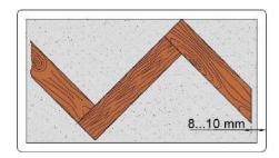
Use a protractor to determine the length and angle of the cut of the last board in a row. Make sure that the length of the adjoining board is sufficient to form an expansion gap after its installation.
