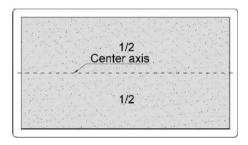
Divide the room in half lengthwise. Mark the center line using chalk line or a laser level to ensure accuracy. Check that the line is straight and aligned with the desired marks. If necessary, secure the line with a permanent marker.
