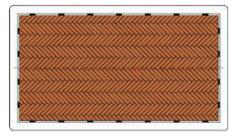
Continue laying to the opposite wall, remembering to install spacers along the walls. Once installation is complete, use the remaining pieces of parquet cut at the beginning. Clean the parquet from debris and dust using suitable care products.
