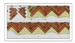
Install spacers along the wall to create a compensation gap. Apply glue to the base. Start laying the boards from the center line, alternating rows on both sides of it. Tap the boards with a hammer through the spacer so that the tongue fits tightly into groove, without gaps.
