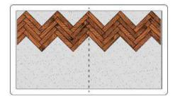
Lay out four or five rows of parquet in the same way as the first. Make sure that each row is laid out evenly and fits tightly against the previous one. Check regularly for proper installation and expansion gaps. Make sure that everything is flat.
