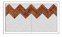
Draw a line with a marker using a straightedge set exactly at the tops of the inside corners of the first row of planks. This will be the starting line after the boards are cut and laid into the overall covering. Number the boards to avoid mistakes when laying them out. Cut the boards along the markings. Use
